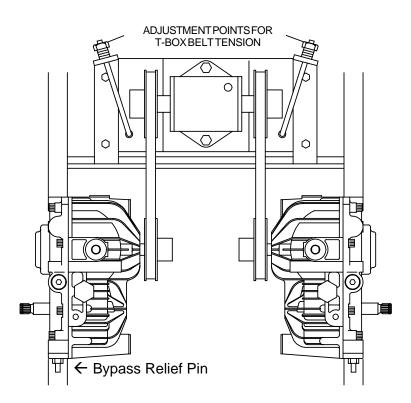
Each hydrostat has a bypass relief pin located at the rear of the hydrostatic unit. A bypass keeper is provided to allow the mower to be rolled around without engine running. To accomplish this, the bypass keeper springs must be positioned to depress the bypass relief pins. Remove bypass keeper springs prior to actual operation of the mower.
